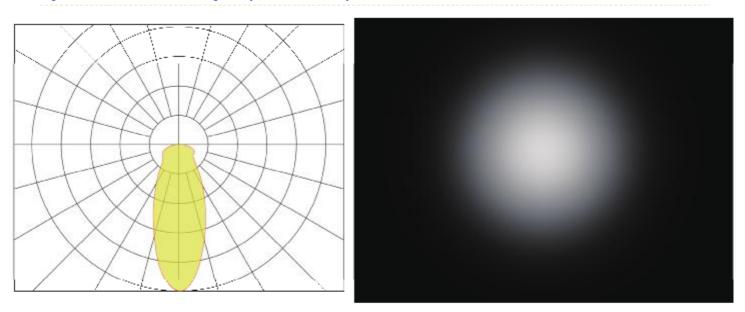
Note: The LED emitter flux is 120lm @350mA
